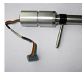
High speed AC electro spindle operating at 60.000 rpm with 11 kW of power and rated torque 1,8 Nm.
